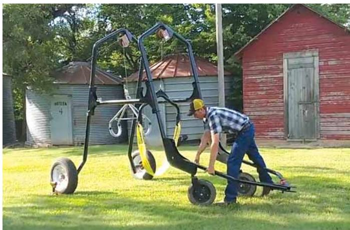
Wheeled sling lift is equipped with a multi-position tongue that hooks up to any pickup bumper.
