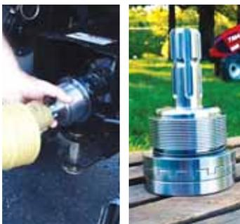
PTO Connect makes connecting an implement to a tractor easier, by removing the radial splines and replacing them with axial splines.
