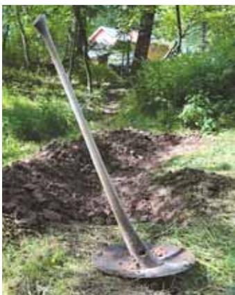
Swinging disk hoe was made by bolting a big coultter onto the end of a 45-in. hickory handle.
