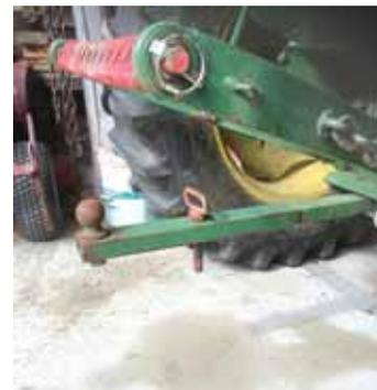
Photos show the "slide-on" trailer ball hitches Reay made for his Ford (left) and Deere tractors.
