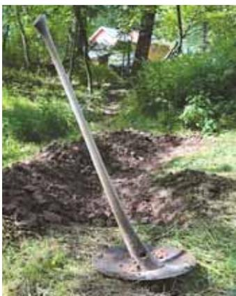
Swinging disk hoe was made by bolting a big coultter onto the end of a 45-in. hickory handle.
