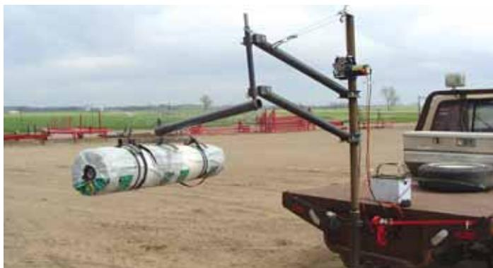
Pickup-mounted, winch-operated lifting device lets one man easily lift a roll of net wrap into balers.
