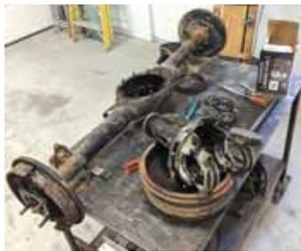
**Rick Bown needed to reverse the pto on a salvaged trash pump he wanted to use as an irrigation pump. So he created a shaft-reversing gearbox by using a piece of 6-in. dia. pipe and a set of spider gears off the rear end of a 1959 Austin car. He stuck the spider gear housing inside the pipe and also cut the axle shafts on the spider gears down to extend past the pipe.**
