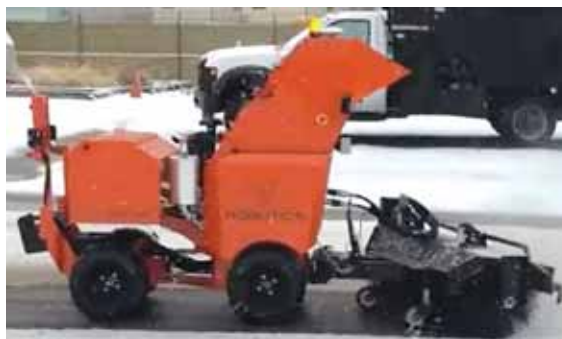
Robotic mower and snow sweeper has on-board cameras that detect obstacles and also allow remote observations by operators.
