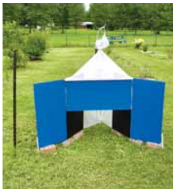
Flies that enter cloth trap are drawn to sunlight at the top, then channeled into a bottle where they die from exposure.
