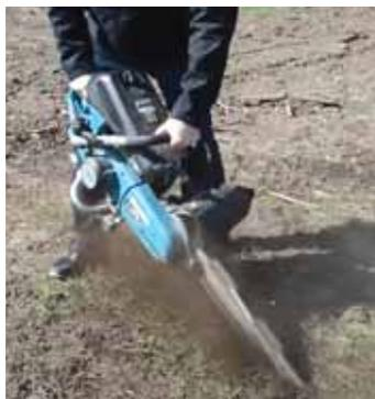
**Handheld GeoRipper can cut trenches up to 16 in. deep and chip through roots up to 3 in. in diameter.**
