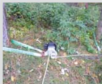
**Battery-powered capstan winch has 2,200 lbs. of pulling power.**
