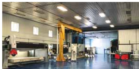
Jeff Hoeft converted his farm shop to build customized countertops out of stone slabs, using an Italian-made computerized CNC saw to cut the stone.
