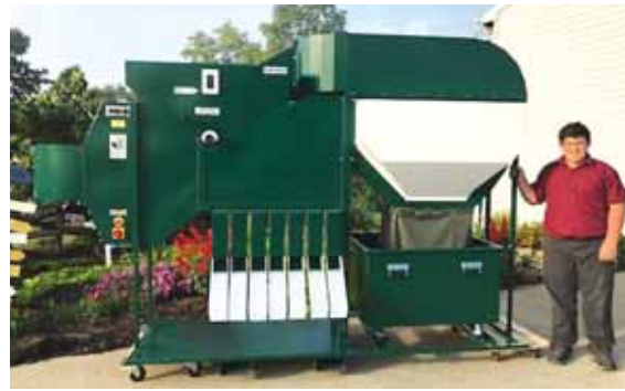
Kharkov ISM (Impeller Separator Machine) uses airflow to separate grain and other materials by their aerodynamic properties.
