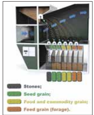
Grain is separated into seed-quality grain, food and commodity grain, and feed grain. Heavy objects such as stones drop out.
