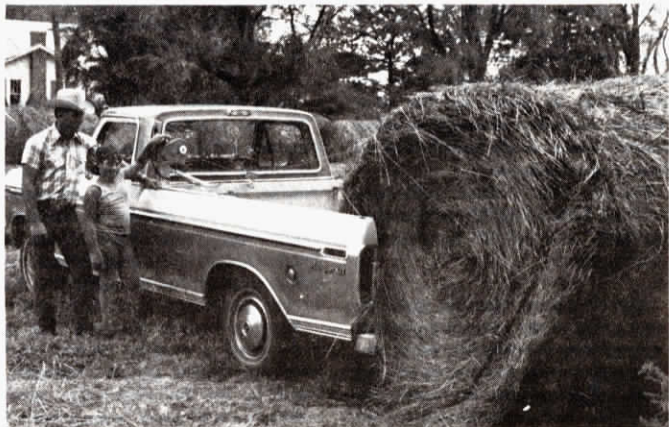
Freck and son load a bale with their "sling" loader. Cable runs from winch to a pulley at front of box and over top of bale.
