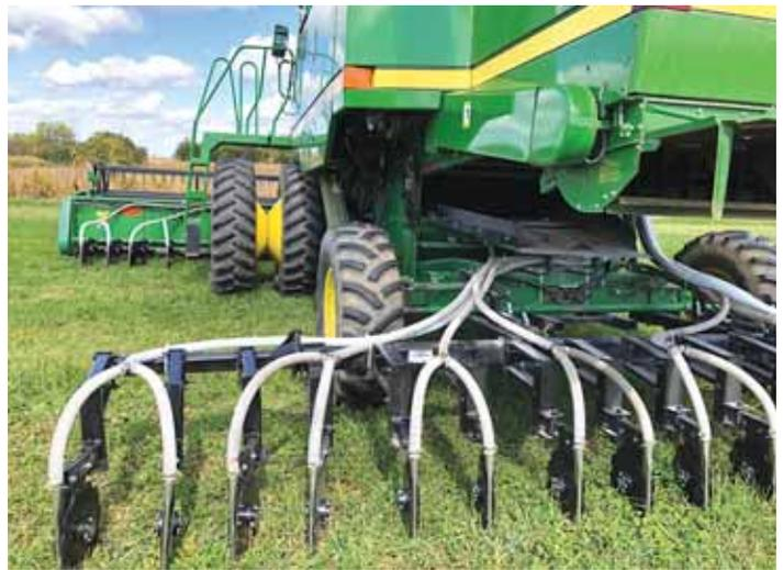
A 15-ft. toolbar with single disc coulters mounts on combine's rear axle, with 6-ft. toolbars mounted to each end of the 30-ft. soybean header.
