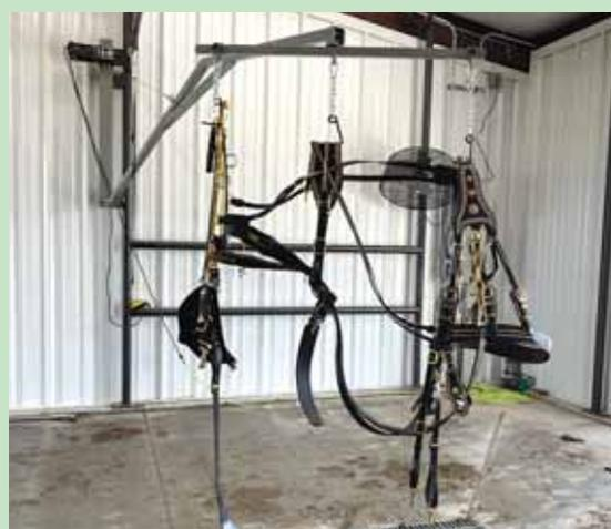
Electric-operated crane extends 15 ft. from barn wall and supports a 4-ft. bar, which has 3 hooks on it to support the harness.
