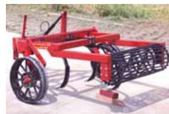
**D.H. Welding modifies horse-drawn stalk choppers (left) and chisel plows for use with compact and small utility tractors.**
