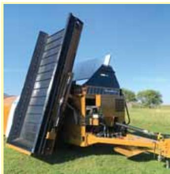
**Pto-operated RamPack silage bagger uses dual plungers to fill plastic forage bags, instead of a rotor or auger. A flywheel and plunger reduce the power needed.**
