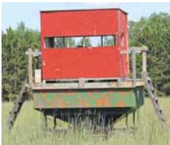
**Crampton mounted a 4 by 8-ft. plywood box on top of an old gravity flow grain wagon to make this mobile deer stand.**
