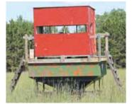
Crampton mounted a 4 by 8-ft. plywood box on top of an old gravity flow grain wagon to make this mobile deer stand.
