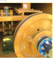
Pto-operated RamPack silage bagger uses dual plungers to fill plastic forage bags, instead of a rotor or auger. A flywheel and plunger reduce the power needed.
