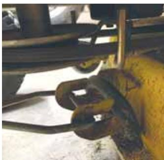
James Minix used rubber tubing to keep the front arm in place on his Deere lawn tractor when mowing over rough ground.
