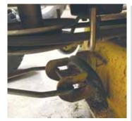
James Minix used rubber tubing to keep the front arm in place on his Deere lawn tractor when mowing over rough ground.
