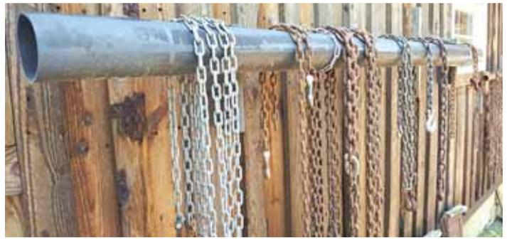
Plastic pipe chain holder is suspended about shoulder high along the wall outside Boggs's shop, making it easy to find the right-sized chain.
