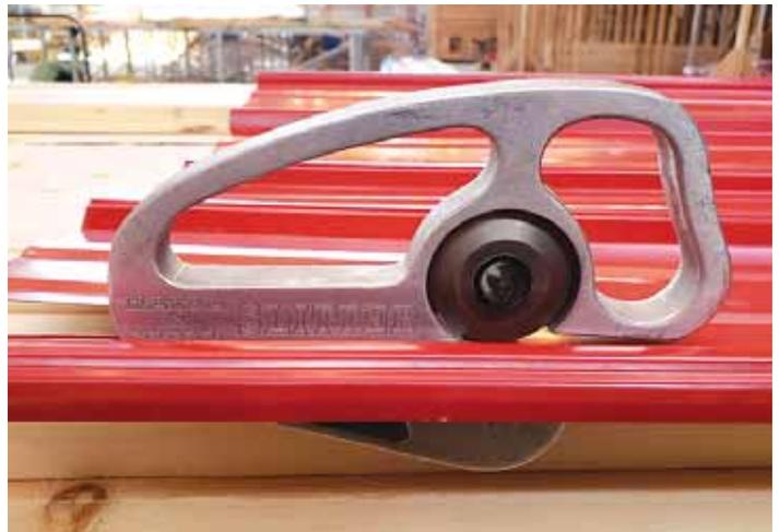
Handheld "slitter" uses a pair of overlapping 2-in. dia. cutter wheels to cut through metal up to 24-ga. thick.
