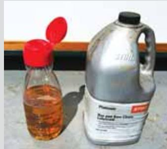
**Doug Johnson, Aberdeen, Wash.:** “When pouring bar oil into the small opening on my chainsaw from the gallon jug it comes in, trying to ‘hit the hole’ often results in spilled oil all over me and the saw. I found that pint-sized Coffee Mate creamer bottles have a good lip for easier pouring, and they’re fairly sturdy plastic bottles. The attached lid snaps in place pretty securely, which is handy when you throw the saw, gas can, and oil into the back of a Gator or pickup. It makes it much
