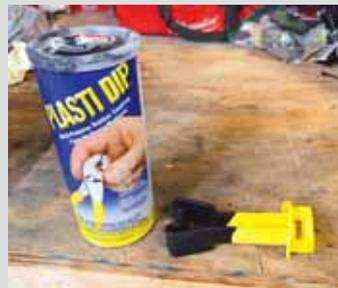
**James Minix, Morrison, Tenn.:** “I was having trouble keeping plastic electric fence insulators from breaking prematurely on chain link fence due to sunlight causing them to get brittle and weak. So I got the idea to protect them by coating the end of the connector that attaches to the fence with Plasti Dip that people normally use to coat handles on shop tools. It seems to work well, extending the life of the insulators by protecting the plastic from the sun.”
