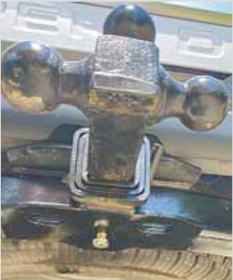
**Larry Wood, Waldo, Ohio:** “Tired of your trailer making noise when you travel down the road? I have a Ford F-350 with a 2 1/2-in. receiver hitch so I use a sleeve adaptor so our 2-in. ball hitch will work properly. But each time I pulled the 2-in. hitch out to change the ball size, the sleeve would move and pinhole would be misaligned.”
