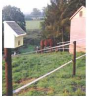
Shock Box has room for a charger and a 12-volt deep cycle marine battery. A solar panel controller attaches to lid.
