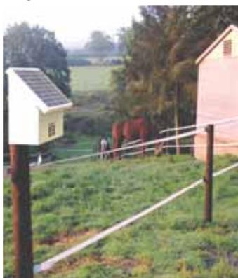
**Shock Box has room for a charger and a 12-volt deep cycle marine battery. A solar panel controller attaches to lid.**
