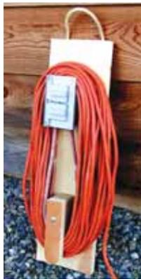
**Cord caddy mounts on a board with an outlet box at one end. Female end of cord is hard-wired to outlet.**
