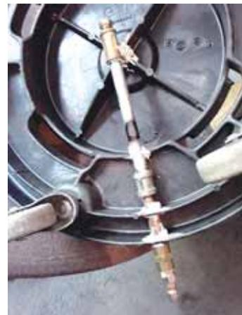
**Plastic wheeled platform off bottom of a rolling trash bin is fitted with a galvanized pipe that hooks up to a pressure washer.**
