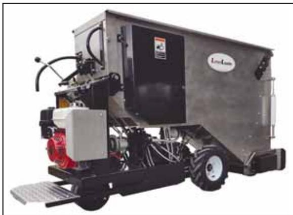
Self-propelled cleaning cart has an auger on front that gathers litter and feeds it to an apron, which carries it up and into hopper.
