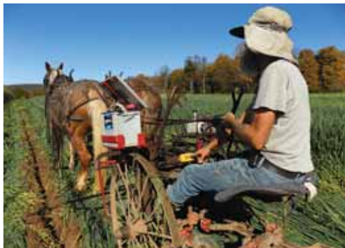
Eric Nordell upgraded his horse-drawn cultivator by adding a hydraulic lift powered by a solar panel, battery, and 12-volt hydraulic pump.
