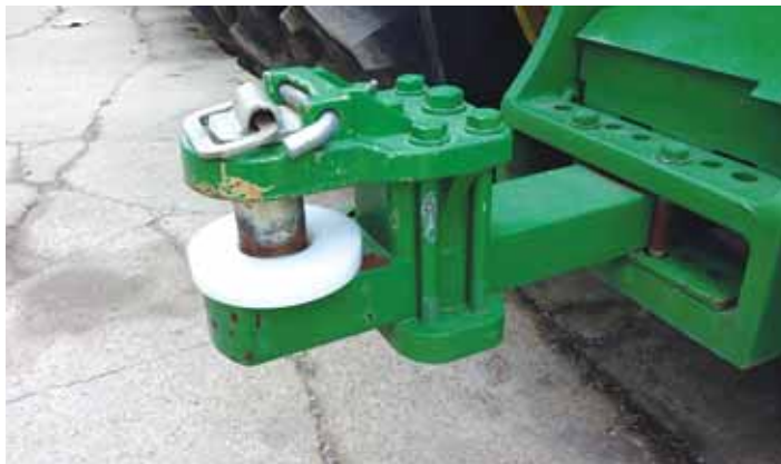
Heavy-duty poly pad installs between hitch and drawbar to reduce wear and tear, says Agassiz Fabrication.
