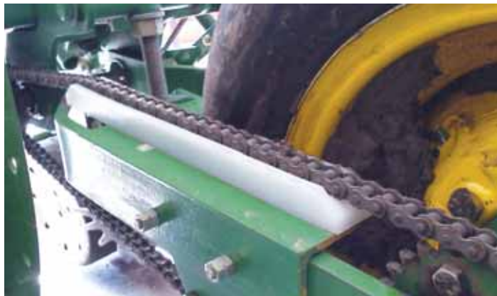
Poly chain guides provide better alignment and reduce wear on planters.
