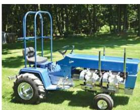
Garden tractor puller is powered by four 8 hp. Harbor reight Predator V-twin engines.
