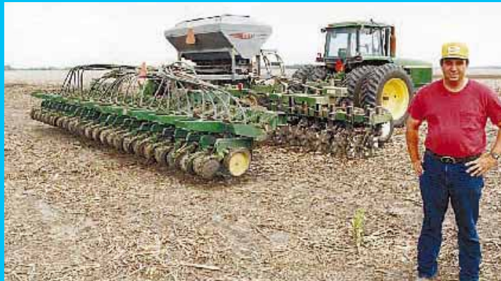
Sam, Bob & Roger Ellis mounted 24 stripped-down Max-Emerge row units on a home-built toolbar and hooked them up to a Hiniker air seeder to plant soybeans.
