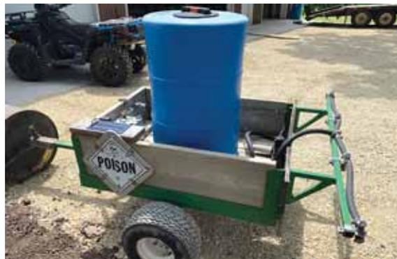
Sprayer cart is equipped with a 50-gal. poly drum and a 4-ft. wide spray boom mounted on back.
