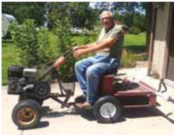
**Sieber replaced walk-behind tiller's tines with wheels, and attached the power unit to a homemade cart.**
