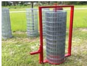
**Bracket slips into a short length of tubing welded onto one side of Ez Fenzer's frame and pins on with 2 bolts.**
