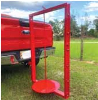
**Ez Fenzer comes with a 2-ft. long, L-shaped "drop hitch" bracket that attaches to fencer and fits into pickup's receiver hitch.**
