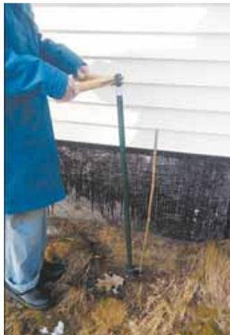
As shears handles are closed together, a threaded rod rotates a curved metal blade at bottom that closes against a grooved metal "stop".
