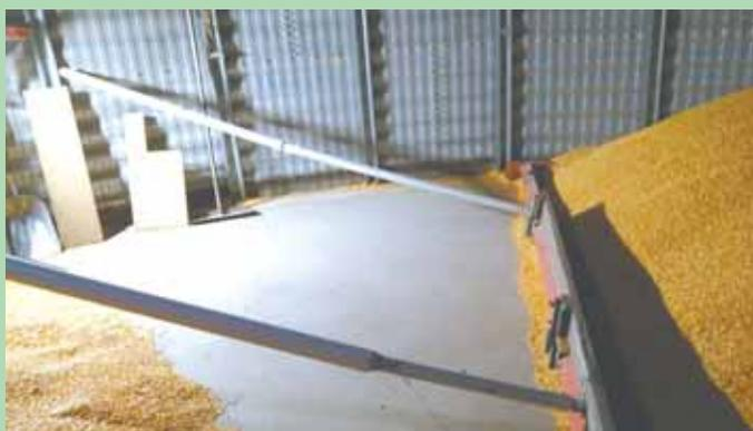
Long pvc "pusher tubes" use spring compression to put constant pressure on bin sweep auger, reducing bin unloading time.
