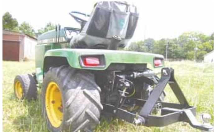
Bill Ruegg says his 3-pt. hitches for Deere lawn tractors work great for plowing, disking, blading and so forth. Photo shows hitch kit on a Deere 318.
