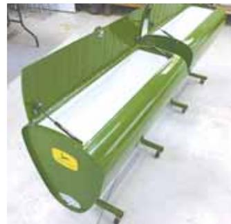
Jim Heitkamp serves up beverages out of a pair of converted Deere fertilizer hoppers. Stands with wheels were welded to the bottom of hoppers, which are lined with styrofoam.
