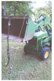
A pair of long ropes are used to open and close log tongs from tractor seat.
