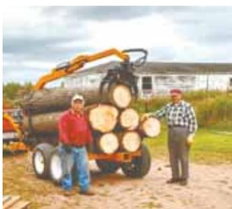
Boom can handle logs up to 8 ft. long by 22 in. diameter.
