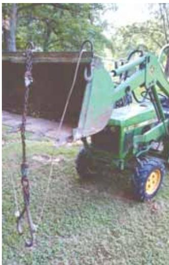
A pair of long ropes are used to open and close log tongs from tractor seat.
