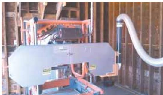
Sawdust collector inside building vacuums sawdust and carries it outside into a covered trailer.
