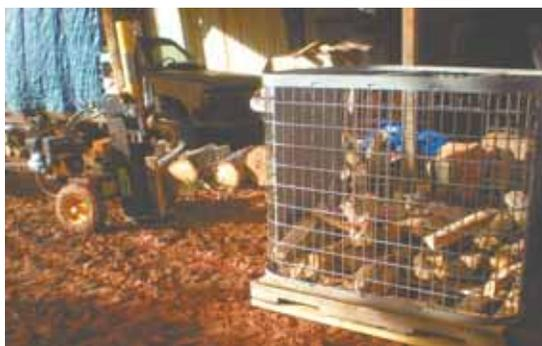
Glenn Fisher converted a pair of 300-gal. metal cage totes to haul and store firewood with less labor.
