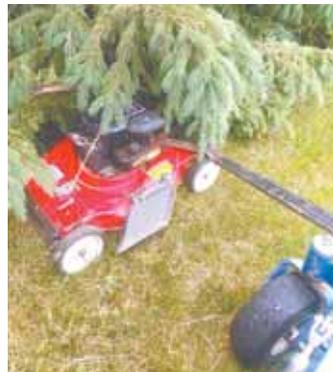
Deflector allows add-on mower to go all the way under lower boughs of evergreens without catching.
