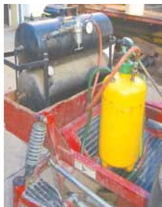
Nahrwald made a pressurized sprayer for his riding mower by plumbing together 2 air tanks from truck brakes, then running an air hose from them to a 3-gal. sprayer.
