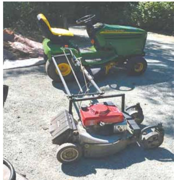
Clutch on side-mount mower lets Drader turn off blades without shutting down engine.
