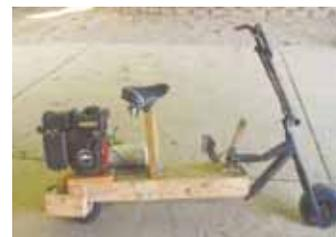
Front end and seat on wood frame scooter came off a bicycle.
