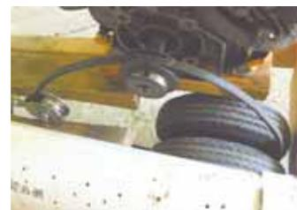
Engine belt-drives a pair of side-by-side rear wheels, with the belt riding between them.
