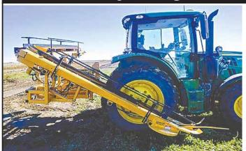
Bish's tractor-mounted, hydraulic-powered hemp harvester cuts the the stalk at ground Bish has adapted its loader-mounted Super Crop header to harvest standing hemp. level and conveys it to a wagon or trailer pulled alongside harvester.
