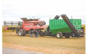
The Grass Hopper, a large wheeled tank, can be pulled behind a combine to collect plant residue. A conveyor delivers material into cart, which unloads it into a truck or trailer at edge of field.
