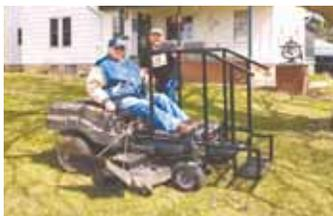
Bottom step is pulled up with a rope to rest on step above it.
