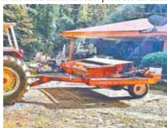
Wilson removed the feeding platform, reel and drum from haybine, then built a stationary hitch and mounted a wheel rake assembly on each side.
