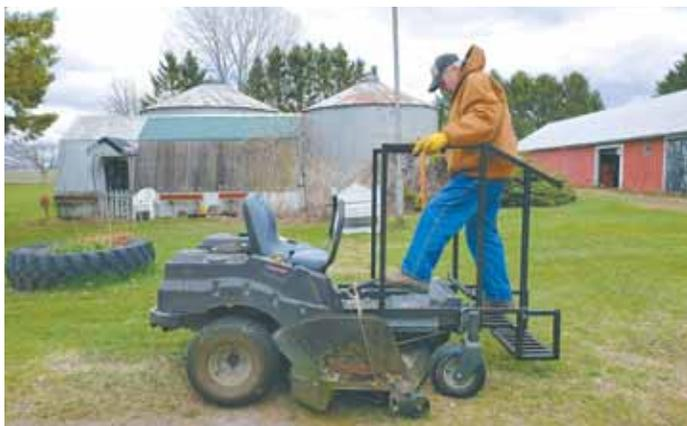
Bob Manzke demonstrates how he uses add-on steps and handrails, built by son Russ, to climb onto mower deck.
