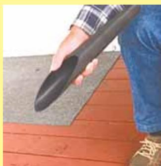
Smith cut the end off a 2-in. dia. leaf blower nozzle at a 20 degree angle. The curvature of the pipe works like a shoehorn.
