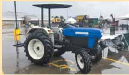
Solectrac's eUtility tractor is designed to replace a 25 to 40 hp. tractor. It has a run time of 5 to 8 hrs. Quick-change battery packs are available.
