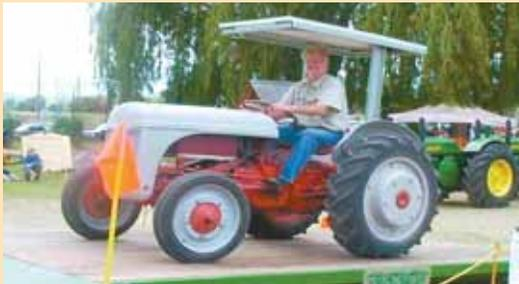
Jerry Clermont's tractor is powered by a 10 hp. electric motor, with four 6-volt batteries recharged by a 24-volt solar panel mounted on an overhead frame.
