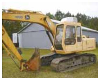
An air conditioning unit from an old motor home keeps the cab cool on Ron Heidebrink's 1988 trackhoe.
