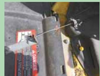
Foot pedal lets Earl Line lift and lower the flap on his mower's grass discharge chute with his foot. Cable runs along mower deck and under the seat.
