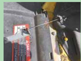
Foot pedal lets Earl Line lift and lower the flap on his mower's grass discharge chute with his foot. Cable runs along mower deck and under the seat.
