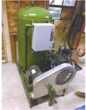
Mark Rinke's customized air compressor rides on a wheeled metal frame and has a shrouded fan, a neatly arranged electrical box, and other accessories.
