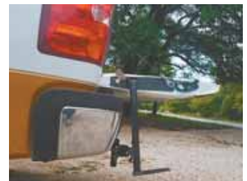
A pivoting tab holds step flat against side of tailgate. You just flip up the tab, pull out the step, and pivot it down into position.
