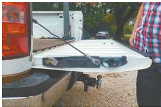
Step is a piece of 1-in. sq. steel tubing with flat metal welded to the bottom. When not in use, it pivots up and then slides inside tailgate.
