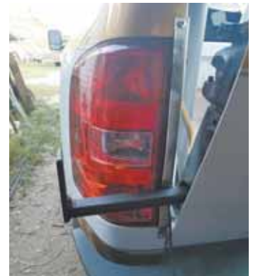
A pivoting tab holds step flat against side of tailgate. You just flip up the tab, pull out the step, and pivot it down into position.
