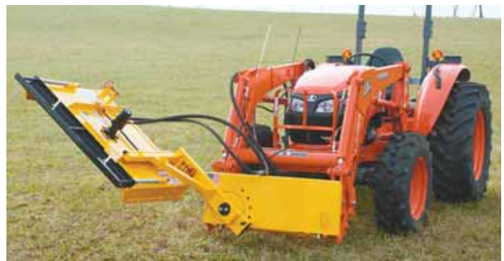
Trailblazer loader-mounted mower comes with a new kind of mount that allows up to 11 different cutting positions.
