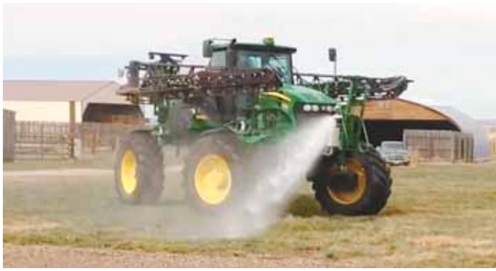
Front turret nozzle on high clearance sprayer can blast water up to 100 ft., fed sprayer's pump and tank.
