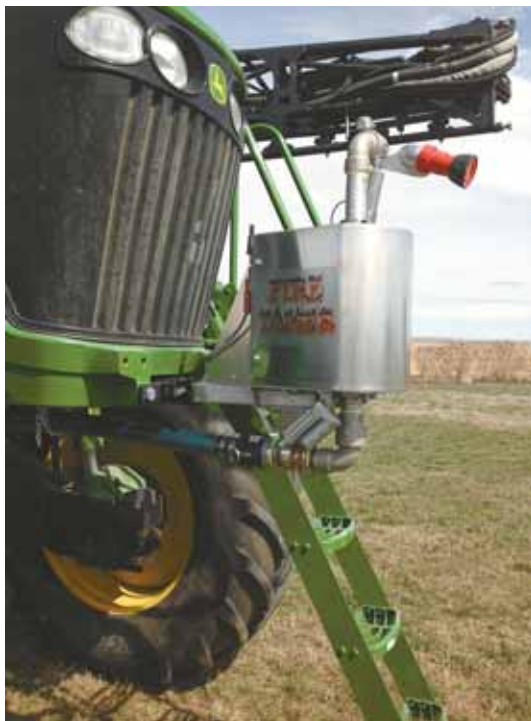
Turret nozzle has 180 degrees of horizontal travel and nearly 70 degrees vertical.
