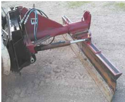
McLae added a hydraulic cylinder to his dirt blade so he can adjust it on-the-go, welding a pivot point for the cylinder base on blade's 3-pt. mounting
