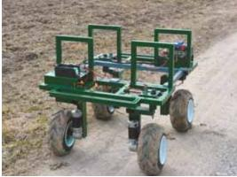
Driverless rabbit tractor can carry a 500-lb. payload while floating across the ground at less than 5 psi. James is developing implements to ride on the work station.
