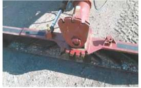
Mirror image brackets welded to either side of blade pivot points are used to and reverse the blade.
