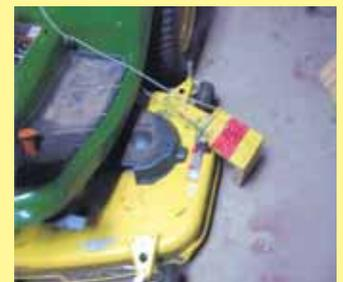
A piece of wood, with a cord attached to it, attaches to a door hinge bolted to mower deck. Yanking the cord flips step up.
