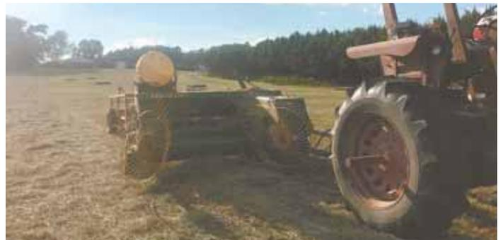
Add-on rake wheels mount on either side of baler pickup.
