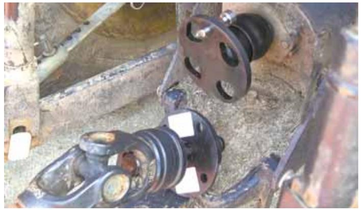
Operator aligns the pieces and runs studs through holes, then rotates male piece. It causes a spring-loaded shear pin on female piece to automatically lock pieces together.
