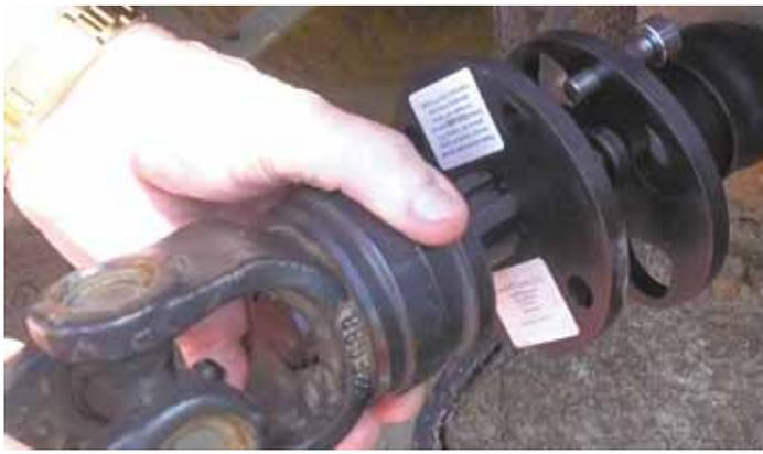
Flat interlocking plate comes in 2 pieces: a male piece with studs that locks onto implement's pto shaft, and a female piece with oblong holes that locks onto tractor's shaft.
