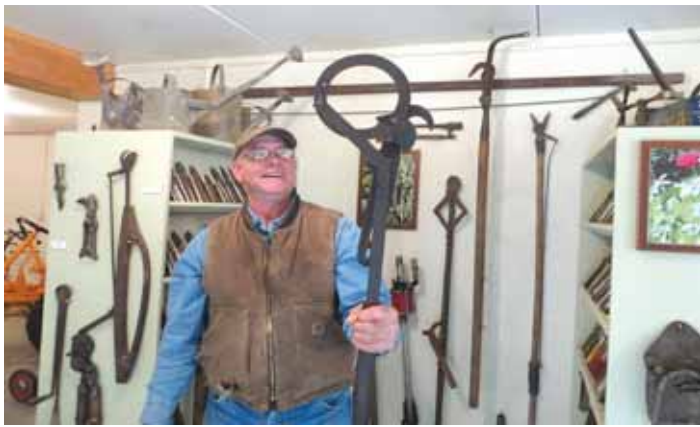
Chuck Witman's garden tool collection includes this unique lopper with a noose that hooks around a tree limb and cuts it as it rotates.
