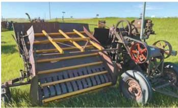
IHC no. 14 baler was built in 1940. It required a driver and a worker with a pitchfork to move the picked-up hay into the bale chamber.
