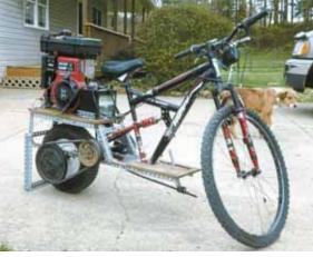
Shawn Wengerd's "tiller" bike" is powered by a 5 hp. rototiller engine on back, which drives a 12-in. all terrain wheel.
