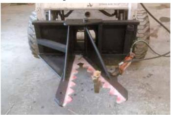
Sawtooth jaws mount on a quick-tach plate, with the left jaw rigid. A hydraulic cylinder opens and closes the right jaw.
