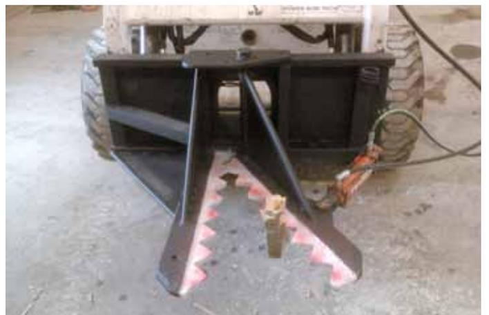
Sawtooth jaws mount on a quick-tach plate, with the left jaw rigid. A hydraulic cylinder opens and closes the right jaw.
