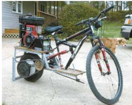
Shawn Wengerd's "tiller bike" is powered by a 5 hp. rototiller engine on back, which drives a 12-in. all terrain wheel.
