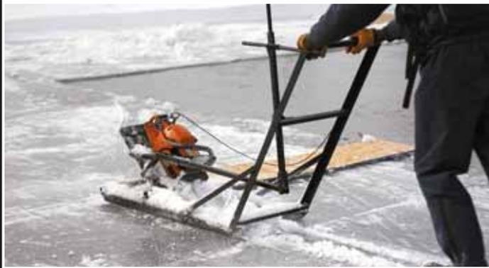
Ice cutter's frame holds chainsaw in place and is pushed backward through the ice. Chainsaw is operated by a remote throttle.
