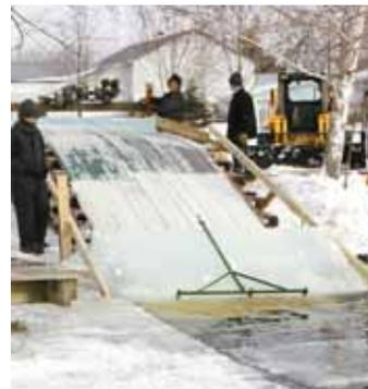
Sheets are grabbed by an ice rake and winched up a ramp and onto a wagon bed. Stacks of ice are then carried to storage by a forklift.
