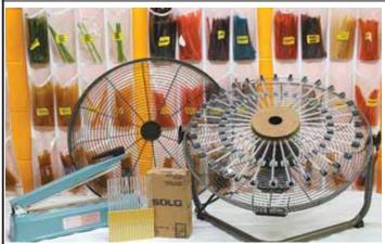
Straws are inserted into 36 holes in perimeter of machine's hub, then filled with honey.
